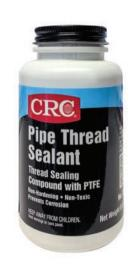
Non-toxic, non-drying thread sealing compound complete with convenient brush top. Engineered to produce a leak-proof seal between pipe thread connections (male and female). Has ability to hold pressures of up to 8000 PSI (55,158kPa). Temperature range -37°C to +287°C. Does not contain lead, graphite, molybdenum disulfide, or clay fillers.
